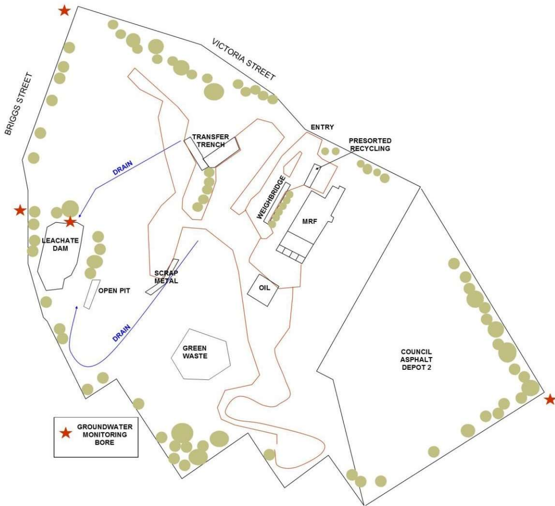
Image 2: Site Plan indicating drainage and leachate dam.
