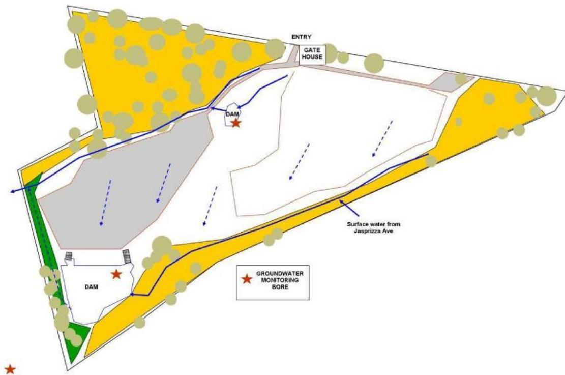
**Image 2: Site Plan indicating drainage and leachate dam.**
