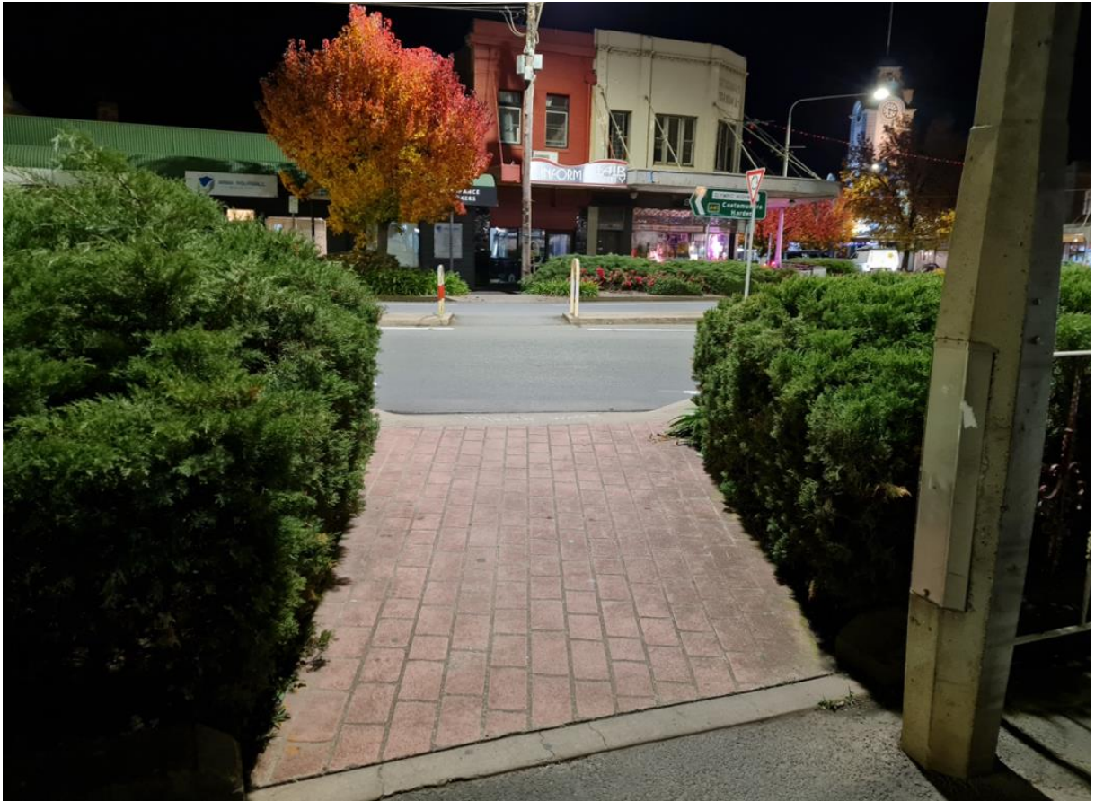
Figure 3.25 Boorowa Street and Main Street roundabout with restricted corner sight distance due to high hedges planted close to crossing.
